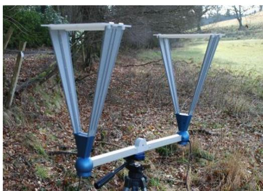
*The two foot foldable bracket is secured to a tripod that uses a standard camera screw mount.
