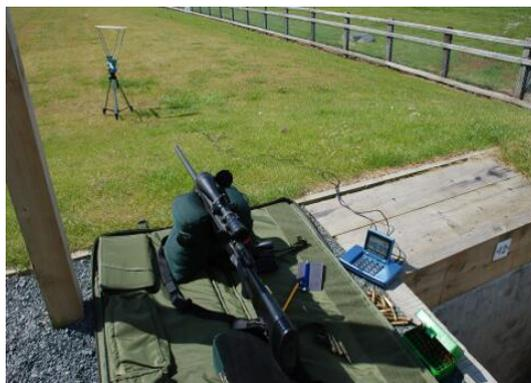
*When measuring the velocity set the screens at maximum cable length so that the muzzle blast does not affect the reading.*
